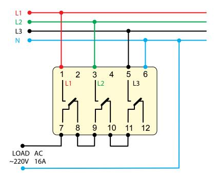
Wiring diagram №2(Magnetic starters-assisted connection under load> 16A (remove jumper straps between the 8-9 and 10-11)
